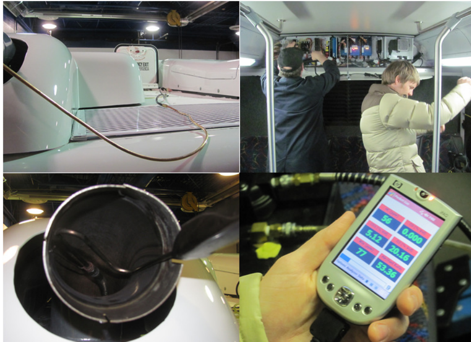
Figure 3. Test set-up. (Clockwise from top left: sample hose position, electrical panel, sample probe inserted, HP handheld display).
